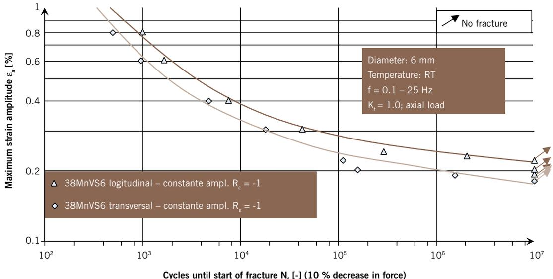
7 The dependence of high-cycle fatigue strength on the orientation of the fibres (Wöhler diagram) [18]
