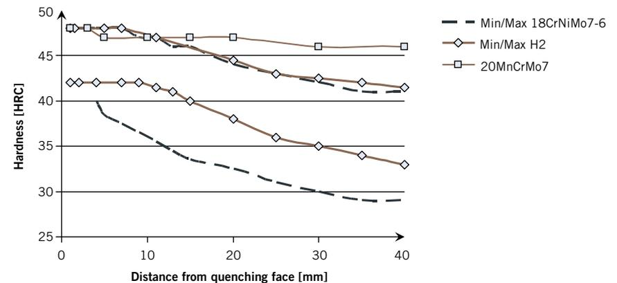
4 Hardenability of two newly developed case hardening steels with cost-effective alloying additions as compared to a conventional highly-alloyed case hardening steel H2
