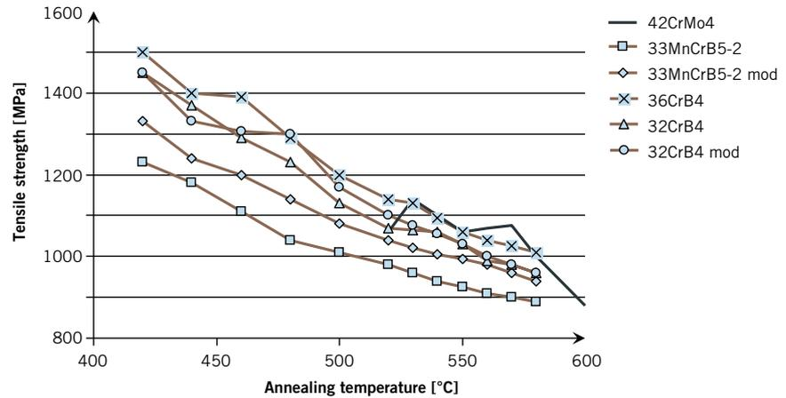
6 Ultimate tensile strength (at room temperature RT) for various molybdenum-alloyed QT steels charted over the annealing temperature [4]
